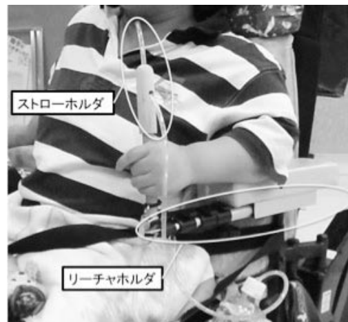
図5 電動車椅子の工夫 Fig.5 Improved wheelchair for using comfortably
