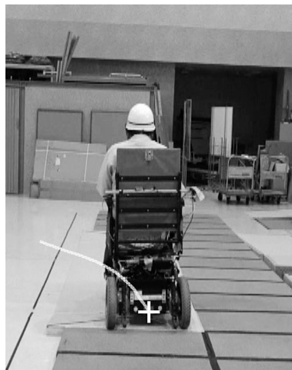
図8 走行実験・制御なし Fig.8 Track on slope without proposed system
