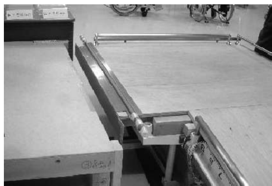
図1 通過実験用段差・隙間架台 Fig.1 Experimental equipment of level difference and gap complex
