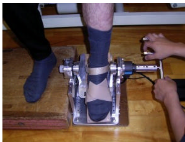
図4 足関節剛性計測の様子 Fig.4 A scene of ankle stiffness measurement
