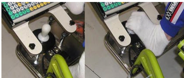
図6 作製したレバー（左）と足によるレバー操作 Fig.6 Operation of the Joystick lever (left) and The joystick using foot (right)
