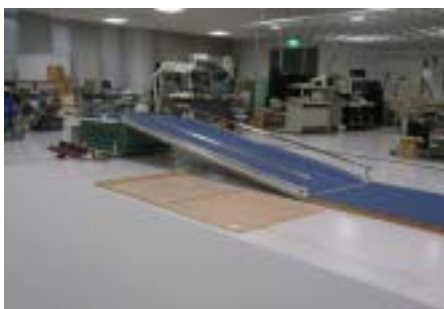
図1 勾配可変試験走行路 Fig.1 Slope track for test running
