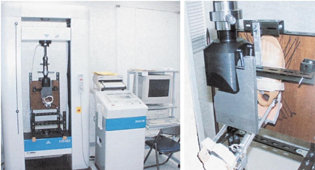
Fig.6 AFO stiffness measurement apparatus
