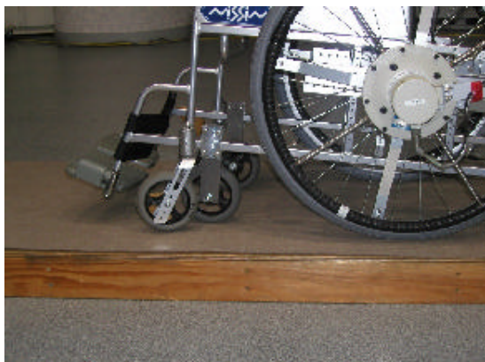
図6 キャスタ機能除去のための固定輪の増設 Fig.6 Set of non-swiveling wheels in place of casters.
