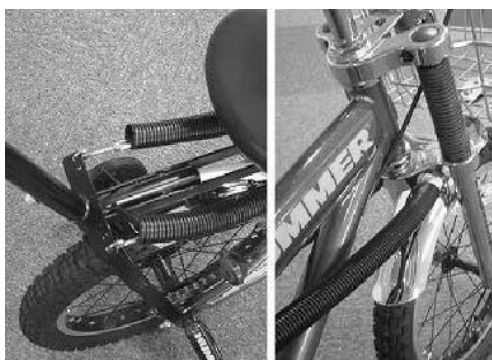
図2 介助用ハンドルの機構 Fig.2 Linkage mechanism of the rear handle to control front wheel direction
