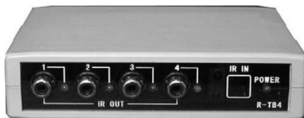
図11 ダイセン電子工業社製学習型リモコン Fig.11 IrDA Learned type remote control device by DAISEN Electric Corporation
