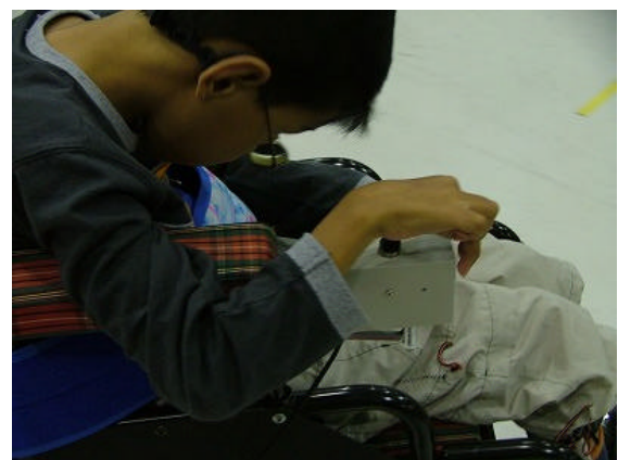
図13 微動電動車いす制御ユニット Fig.13 System for cerebral palsy to run a wheelchair while several seconds by pushing a switch
