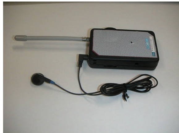
図6 タグの検知器 Fig.6 Detector of tags for a wandering system
