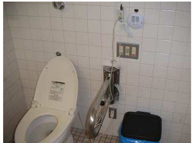
図10 トイレ立ち上がり検知センサ Fig.10 Sensor being aware of the presence of standing up from a toilet seat
